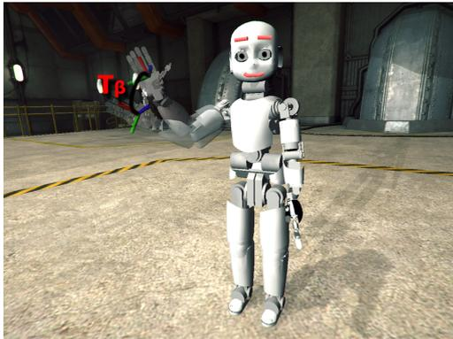
Fig. 13: Cartesian error transformation matrix ( $T_{\beta}$ ) between the real hand pose and the hand pose estimated by using the robot model.
